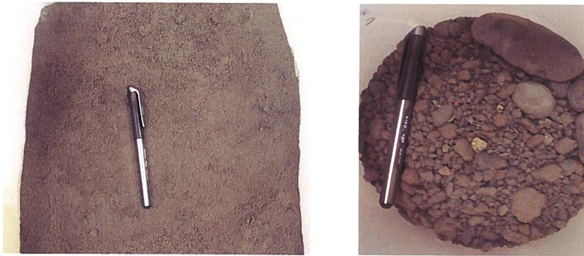
Figure 2. Hanford sediment passing No. 18 sieve (left) and retained on No. 18 sieve (right).
