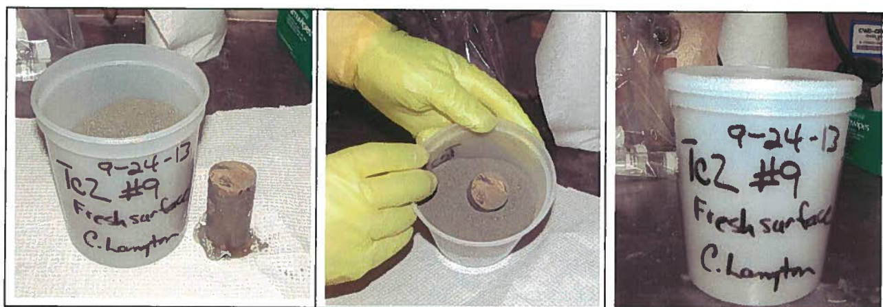
Figure 1. Epoxy coated sample with uncoated top surface, soil leaching media before sample was covered with about 3 cm of additional sediment, and container during exposure.
