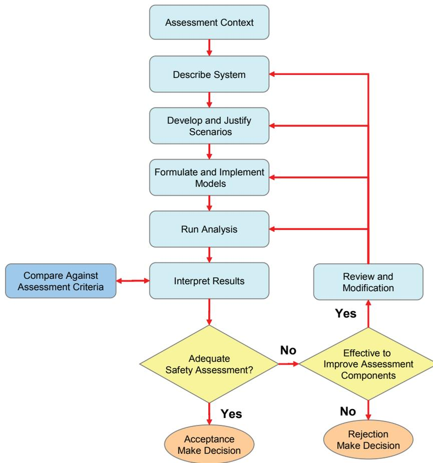
**Figure 2. Example of Safety Assessment Methodology (after IAEA 2004)**
