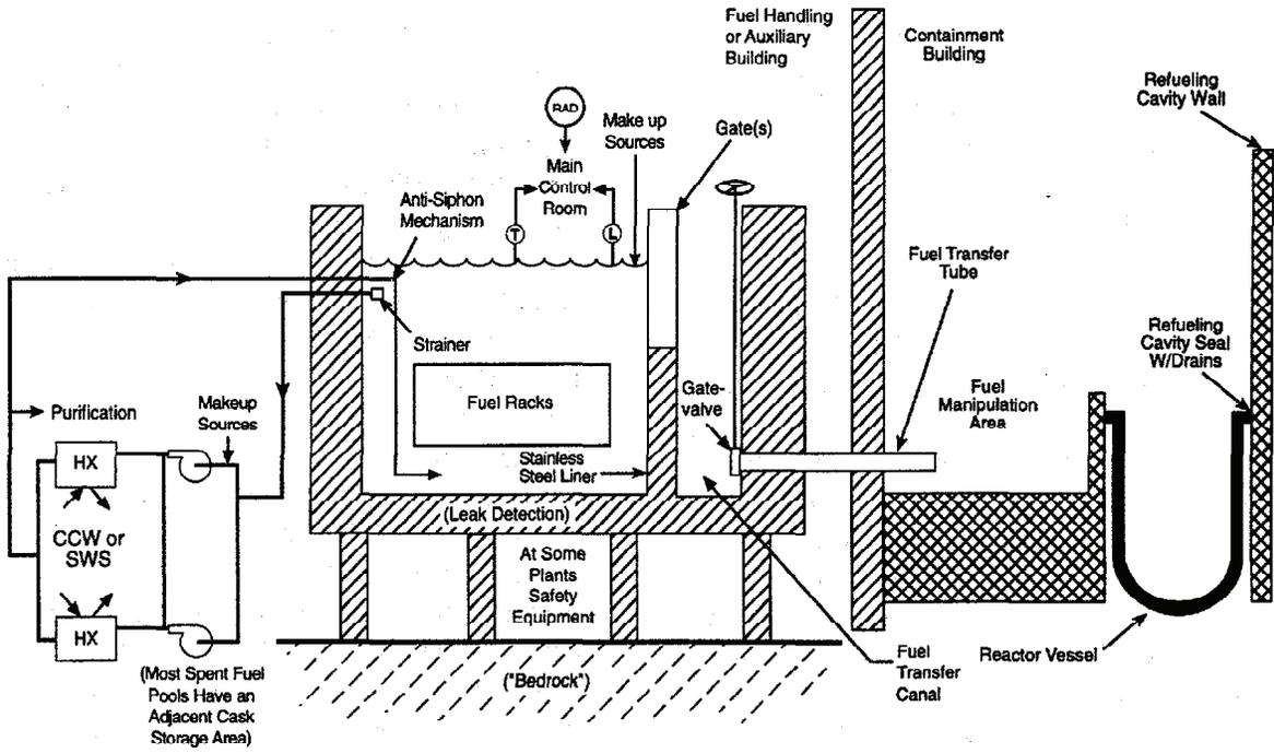
Figure 22. Pressurized Water Reactor (PWR) Spent Fuel Cooling Systems
