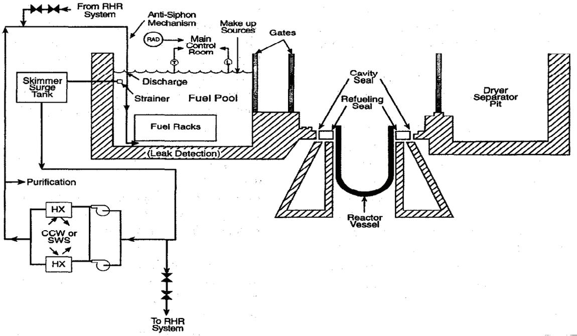
Figure 21. Boiling Water Reactor (BWR) Spent Fuel Cooling Systems
