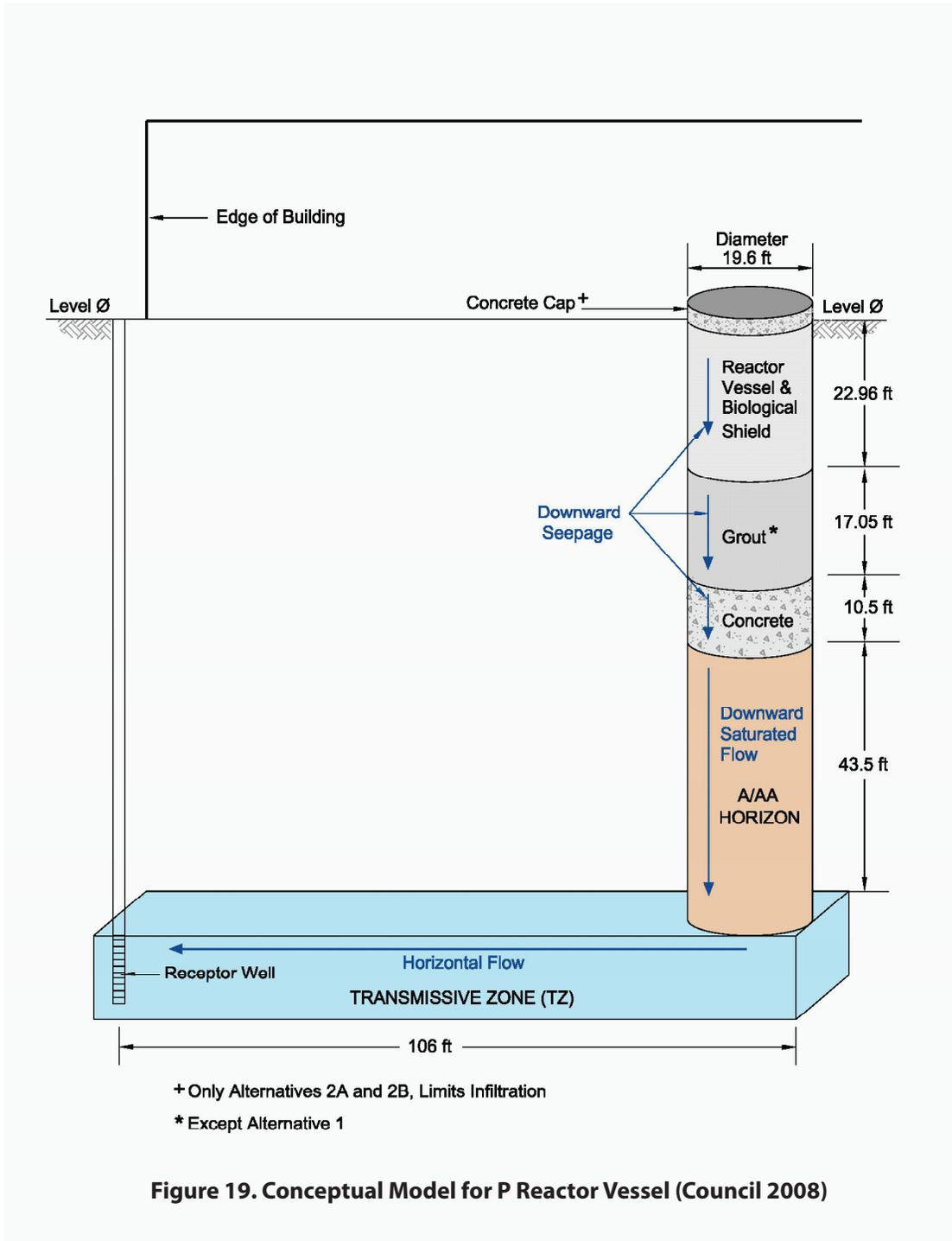
Figure 19. Conceptual Model for P Reactor Vessel (Council 2008)
